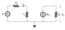
$$\frac{V_0}{V_s} = \frac{-\beta I_b \times R_L}{I_b (R_s + r_\pi)}$$
