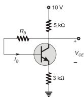
If  $I_B$  = 10  $\mu$ A and  $\beta$  = 100, then  $V_{CE}$  is \_\_\_\_\_
