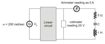
Then the value of capacitor 'C' is  $\_\_\_$   $\mu$ F.
