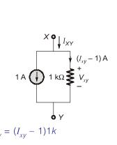
$$V_{xy} = (I_{xy} - 1)1k$$
