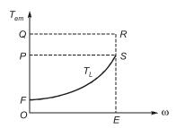
The shortest time will be taken if motor follows the path that maximize the net accelerating torque (Tem- $T_I$ ) at all points.
