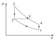
For same compression ratio and same heat rejection, heat supplied is maximum in Otto cycle, then dual cycle and minimum in diesel cycle.
