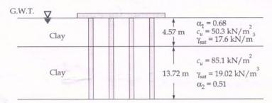
The piles are square in cross-section (356 mm  $\times$  356 mm). The center-to-center spacing, d of the piles is 889 mm. Determine the allowable load carrying capacity of the pile group. Use FOS = 4.
