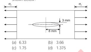
Q.2 In the given diagram, high cycle fatigue starts from
