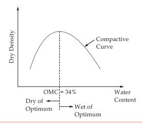
Given : Moisture content = 30% (< OMC)  $\Rightarrow$  Dry of optimum Hence, structure after compaction will be flocculated.
