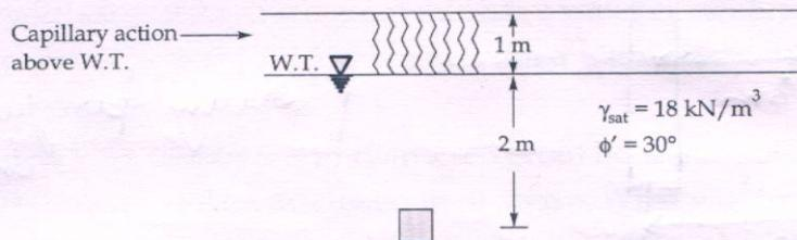
The soil is a homogeneous, poorly graded sand. Determine the increase in vertical effective stress at which a soil element at a depth of 3 m, under the center of the building will fail if the increase in lateral effective stress is 20% of the increase in vertical effective stress. The coefficient of lateral earth pressure at rest  $k_0$  is 0.5. [Assume all stresses are principal stresses.]
