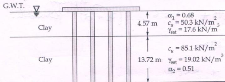
The piles are square in cross-section ( $356 \text{ mm} \times 356 \text{ mm}$ ). The center-to-center spacing,  $d$  of the piles is 889 mm. Determine the allowable load carrying capacity of the pile group. Use FOS = 4.
