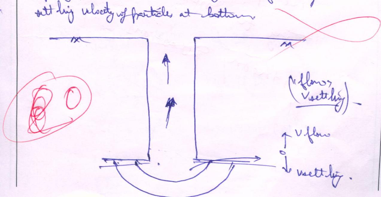
As the velocity of flow increases, thereby, the base of the well is disturbed and ultimately the well sinks in. This sinking in of well is termed as sinking of well. If this problem isn't rectified in a short duration of time, the storage capacity of a well can reduce by a large amount. Thus, it is important for the engineer to properly seal the wall of the well so that cavity doesn't develop.
