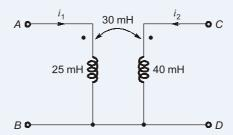
Establish the equivalence between the network and its *T* equivalent.
