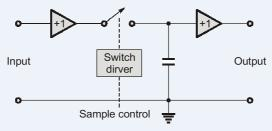
$A_1$  is an input buffer amplifier with a high input impedance so that the source, which may be an analog multiplexer, is not loaded. The output of  $A_1$  must be capable of driving the hold capacitor with stability and enough derive current to change it rapidly. S<sub>1</sub> is an electronic switch, generally an FET, which is rapidly switched on or off by a driver circuit that interfaces with TTL inputs.
