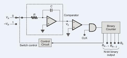
The basic operation of this ADC involves the linear charging and discharging of capacitor 'C', using constant currents.
