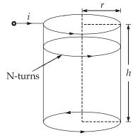
(i) For the direction of current *i* shown in figure above, the magnetic field inside the solenoid is directed axially upward.
