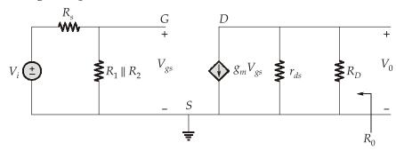
$$r_{ds} = \frac{1}{\lambda I_{DQ}} = \frac{1}{0.01 \times 1.059 \times 10^{-3}}$$
