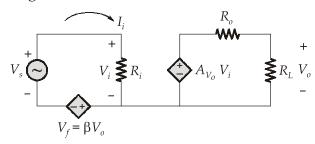
where,  $R_i$  = Input impedance without feedback  $R_o$  = Output impedance without feedback  $A_V$  = Voltage gain for finite ' $R_L$ '  $A_{V_o}$  = Voltage gain for infinite ' $R_L$ '
