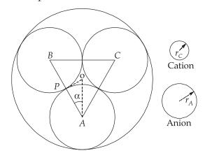
This boils down to a relatively simple plane trigonometry problem. Consideration of the right triangle APO makes it clear that the side lengths are related to the anion and cation radii  $r_A$  and  $r_C$  as
