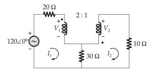
Applying mesh analysis for mesh - 1,
