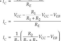
The maximum allowable value of  $R_C$  is obtained by equating the base and collector voltages. For  $R_C > R_{C \text{ max}'}$  the transistor operates in saturation region as  $V_C > V_B$ .
