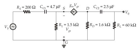
Calculation of time constant  $(\tau_1)$  associated with  $C_{C1}$ :
