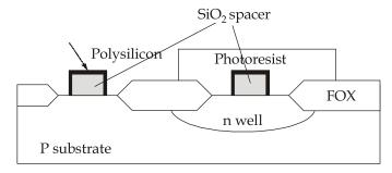
Step 8: Implantation of NMOS source and drain and contact to n well (not shown).
