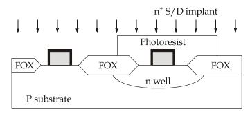
**Step 9:** Remove sidewall spacers and implant the NMOS lightly doped source/drains.
