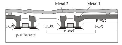
**Step 15:** Etch unwanted metal and deposit a passivation layer and open over bonding pads.
