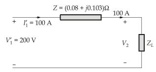
(a) Voltage drop for 0.8 pf lagging load is 12.58 V
