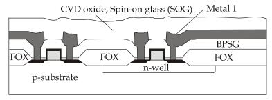
**Step 14:** Deposit another interlayer dielectric (CVD SiO<sub>2</sub>), open contacts, deposit second level metal.
