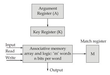
The argument register A and key register are of *n* bits. The match register has M bits each for one memory word. Each word in memory is compared in parallel with content of argument register. The words that match the bits of the argument register set a corresponding bit in the match register. After the matching, those bits in match register that have been set indicate the fact that their corresponding words have been matched.
