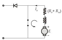
$$E = I_a(R_a + R_{se}) = 60 \times (0.15) = 9 \text{ V}$$
