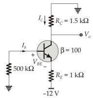
$$g_m = \frac{I_C}{V_T} = \frac{1.88 \text{ mA}}{26 \text{ mV}} = 72.31 \text{ mA/V}$$
