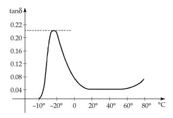
At low temperature, the loss due to dipole polarization is greater than that due to the leakage current. At temperature much below 0°C due to less thermal motion, orientation of dipoles is limited. With increase in temperature the dipoles acquire greater mobility, hence increase in temperature causes the loss tangent to drop off due to enhanced thermal agitation. After falling to a minimum,  $\tan\delta$  begins to increase, this time due to an increase in the leakage current.
