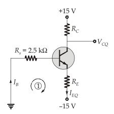
$$I_{CQ} = \frac{\beta}{\beta + 1} \times I_{EQ} = \frac{99}{100} \times 0.5 = 0.495 \text{ mA}$$
