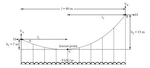
For cable with ends at different levels.
