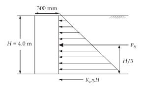
$$k_a = \frac{1 - \sin \phi}{1 + \sin \phi} = \frac{1 - \sin 30^{\circ}}{1 + \sin 30^{\circ}} = \frac{1 - \frac{1}{2}}{1 + \frac{1}{2}} = \frac{1}{3}$$
