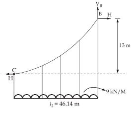
Using free body diagram of cable,
