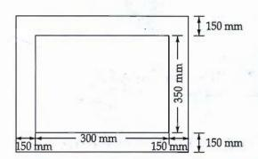
Design the beam as shown in figure for a working bending moment of 285 kN-m using M25 concrete and Fe415 steel and using limit state method. Consider effective cover for all reinforcement as 50 mm.
