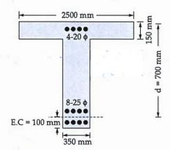
Clear span of T-beam = 10 m.
