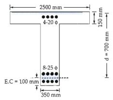
Clear span of T-beam = 10 m.
