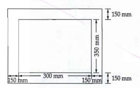
Design the beam as shown in figure for a working bending moment of 285 kN-m using M25 concrete and Fe415 steel and using limit state method. Consider effective cover for all reinforcement as 50 mm.
