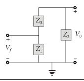
The feedback gain,  $\beta = \frac{V_f}{V_0} = \frac{Z_1}{Z_1 + Z_2}$
