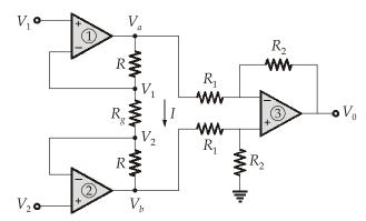
As all op-amps has -ve feedback so current zero concept is applied
