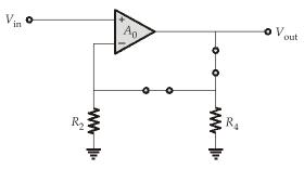
$V_{\text{out}} = V_{\text{i}}$
