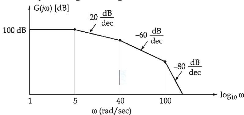
Estimate the magnitude of transfer function at each of the corner frequencies and also calculate the phase margin.
