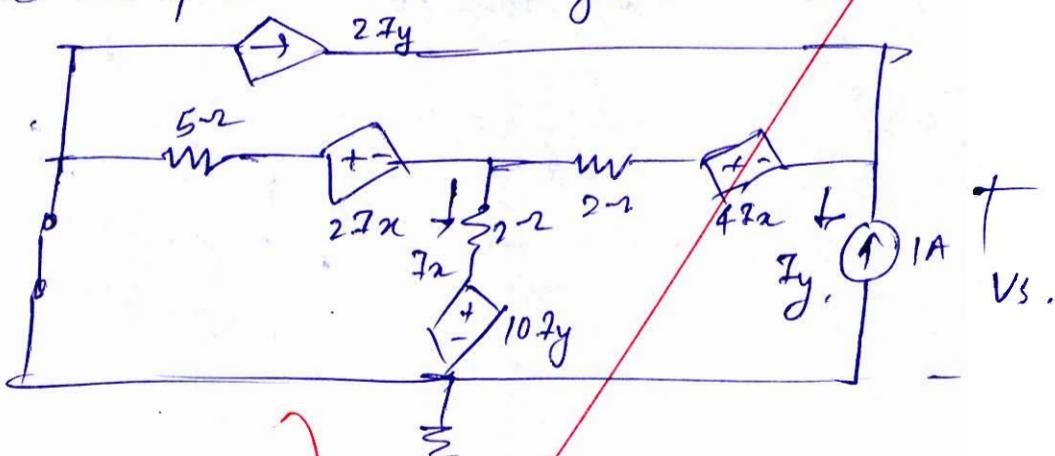
We have connected 1A source to activate the dependent sources hence,  $R_{th} = \frac{Vs}{I}$ .  $\Rightarrow R_{th} = V_s$
