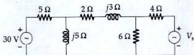
Determine the voltage  $V_b$  which results in a zero current through the  $(2 + j3)\Omega$  impedance branch. Using superposition theorem.
