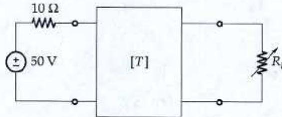
The output port is connected to a variable load for maximum power transfer. Find  $R_L$  and the maximum power transferred.
