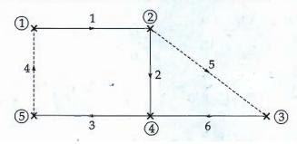
(iii) For the network shown in figure, write down the f-cutset matrix, obtain the KCL equilibrium equations in matrix form and calculate v.
