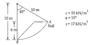
Normal effective pressure on sliding surface AB is 225 kN/m<sup>2</sup>.
