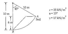
Normal effective pressure on sliding surface AB is 225 kN/m².
