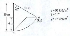
Normal effective pressure on sliding surface AB is 225 kN/m<sup>2</sup>. Downward tangential disturbing force along AB is 850 kN/m.
