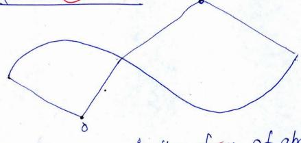
when a curve in the form of above mentioned curve is set it is known as Reverse curve 9n this curve there are Reverse for each side of 2 different centres for each side of twin. But both centres lie on same line
