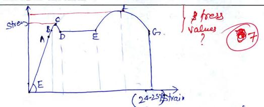
A = Proportional limit - Upto this point straws is directly proportional to strain.
