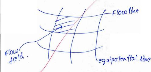
flow field is square for isotrophic and curvilinear square for non isotrophic
