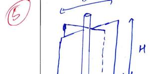
T = Cu TD D + H ) w two sides shearing
