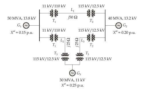
Given: Base:  $MVA_b = 50 \text{ MVA}, V_b = 13.8 \text{ kV}$
