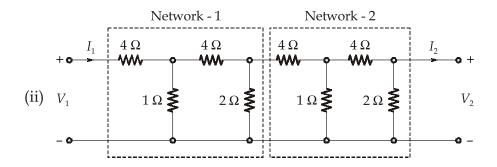
Here, network 1 and network 2 are identical and cascaded.
