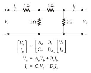
**Case I :** Open circuiting the output port, i.e.,  $I_b$  = 0.
