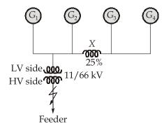
Let the base MVA chosen be 20 and base kV be 11 kV on generator side and 66 kV on feeder side. Per unit reactance of each generator,
