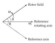
$\omega_r$  is angular velocity of the reference synchronously rotating axis and  $\delta$  is angular displacement in electrical degrees from synchronously rotating reference axis,
