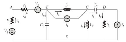
While drawing oriented graph, voltage sources are short circuited while current sources are open circuit. The oriented graph with node E as reference node, and branch currents indicating branch numbers is as shown below.
