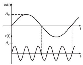
In AM, the instantaneous amplitude of carrier changes in proportion with the modulating signal as shown below.
