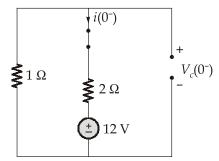
Since, the inductor current and capacitor voltage cannot change instantaneously, we have
