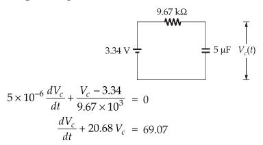
The solution of the above linear differential equation is given by
