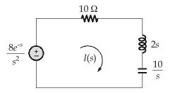
Applying KVL to the Mesh for t > 0,
