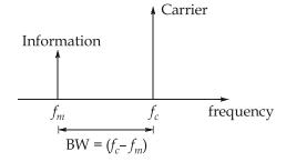
The spectrum of the linear addition as shown in fig. above. It indicates that there is no freq. translation of the modulating signal and the information is contained in the low frequency spectrum.
