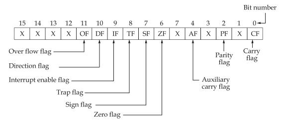
There are nine status flags as shown in figure. Out of the 9 flags, 6 flags are condition flags and remaining 3 flags are control flags. The condition flags are similar to that of 8085 as carry, parity, auxiliary carry, zero, sign and over flow flags. The control flags are direction, trap and interrupt flags.
