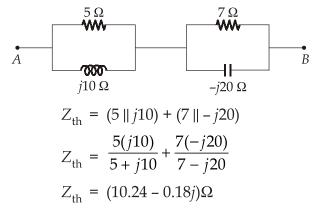
For maximum power transfer, the load impedance should be complex conjugate of the Thevenin impedance,
