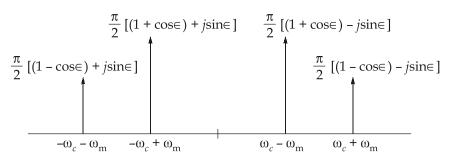
(iii) From equation (i), the power in the desired LSB component at  $(\omega_c - \omega_m)$  is
