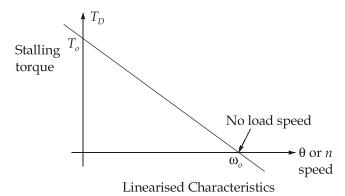
**Calculation of Transfer Function :** The developed torque  $T_D$  is a function of speed and control voltage from the linearized torque-speed characteristics. The equation which relates the torque of the motor and the speed is given by :
