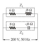
(i) The impedance,  $Z_1 = 6 + j8 = 10 \angle 53.13^{\circ} \Omega$ The impedance,  $Z_2 = 8 - j6 = 10 \angle -36.87^{\circ} \Omega$
