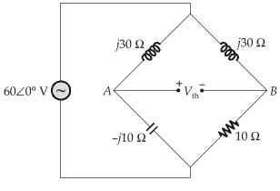
$$V_{\text{th}} = V_{AB} = V_A - V_B$$
