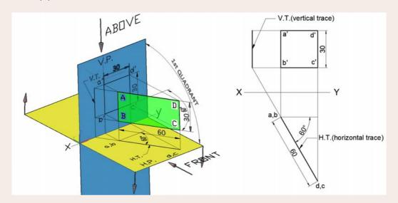
Traces of a plane are defined as line of intersection of plane or plane extended with reference planes or planes of projection.
