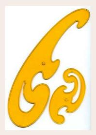
In manual drafting, French curves are used for drawing curves which cannot be drawn by compass. Faint freehand curve is first drawn through the known points. Longest possible curves exactly coinciding with the freehand curve are then found out from the French curve. Finally, neat continuous curve is drawn with the aid of the French curve. Care should be taken to see that no corner is formed anywhere within the drawn curve.
