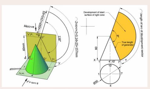
As shown in figure, Radial line development method is used for development of lateral surface of right cone in which the true length of generator is used as radius of development sector
