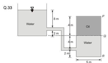
A 5 m × 5 m closed tank of 10 m height contains water, oil and is connected to an overhead water reservoir as shown.
