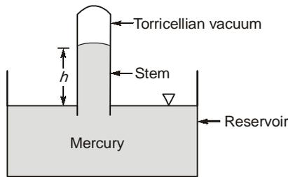
If there is a hole in the vacuum portion, then there will be zero pressure difference at top and bottom of the stem. The mercury in the stem will show zero reading i.e. it will fall and get collected in the reservoir.
