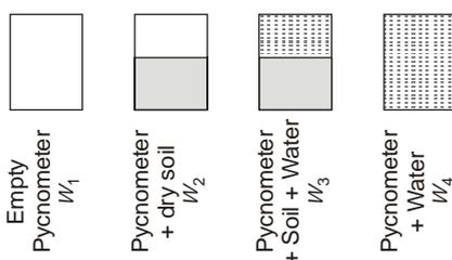
The specific gravity of the solids is given by
