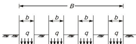
The significant depth  $D_s$ , i.e., depth of vertical stress contour, having a value of  $0.2q$  will be
