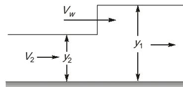
As there is decrease in the depth and increase in velocity of flow after passage of surge so it means the surge is negative and travels downstream.
