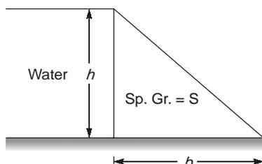
**Reason (R) :** The resultant force will pass through the centroid of the pressure distribution diagram on the base, for the nil or full storage if the ratio
