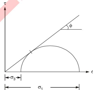
For drained condition,  $\phi$  will be mobilized, for normally consolidated clay failure envelope passes through origin so  $C = 0$ .
