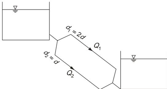
For parallel pipes, head loss is same
