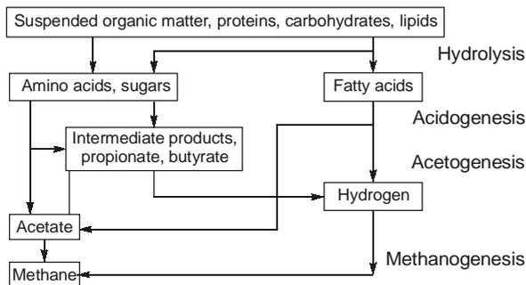
Different steps are necessary for the anaerobic digestion of proteins, carbohydrates, and lipids. Four different phases can be distinguished in the overall conversion process of organic matter to biogas as (1) Hydrolysis, (2) Acidogenesis, (3) Acetogenesis and (4) Methanogenesis.
