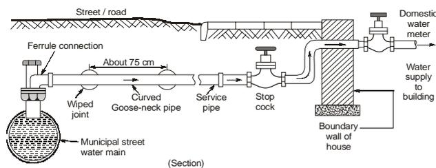
Service connection includes ferrules, stop cock, goose pipe, service pipe, water meters, water taps, bib cocks, spouts, pipe fittings such as bends, crosses, tees, elbows, union, plugs, flanges etc.
