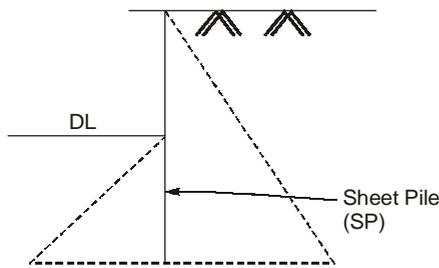
Cantilever Sheet Pile, Cohesive Soil – Approximate analysis
