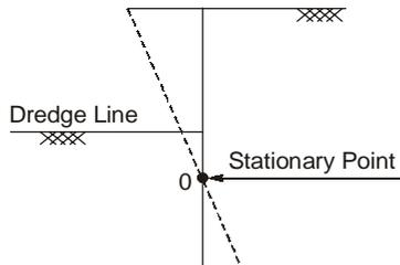
Above the dredge line, the pressure is active on the back of the wall. Near the embedded end the pressure on the back of the wall will be passive as the wall moves towards the fill.
