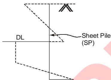
Anchored Sheet Pile, Granular Soil – Fixed Method
