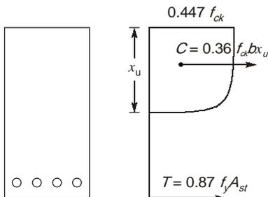
The compressive strength of concrete in the structure shall be assumed to be 0.67 times the characteristic strength. The partial safety factor of 1.5 shall be applied in addition to this. Thus stress in concrete at collapse
