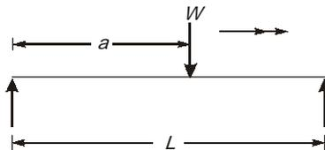
**Reason (R):** When the load maintains the same  $a/L$  ratio in all spans, the reaction at the right hand support remains the same.
