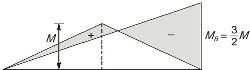
Moment under the load in the beam =  $\frac{M}{4}$
