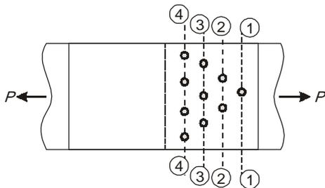
The section 1 – 1 is most critical. The strength of joint at section 1 – 1 is  $(b - d) t \sigma_{at}$ .
