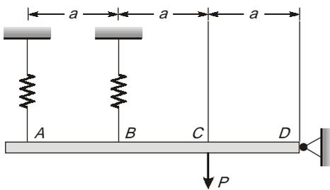
The ratio of forces of spring at  $A$  and that of spring at  $B$  is
