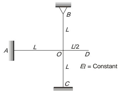
If joint O of the frame is rigid, the rotational stiffness of the frame at point O is given by
