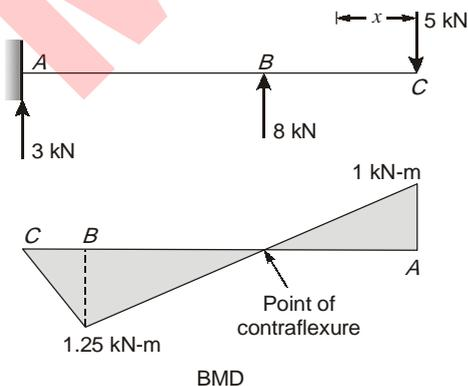
Distance of point of contraflexure from A is  $x$ ,
