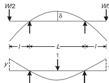
**Reason (R):** The equation for the unknown deflection  $\delta$  from influence line diagram for deflection at mid-span is  $\delta = Wy$ .
