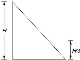
The centre of pressure will lie at  $H/3$  from bottom of retaining wall.
