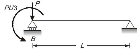
If there was no load on overhanging part the deflection of load point would have been
