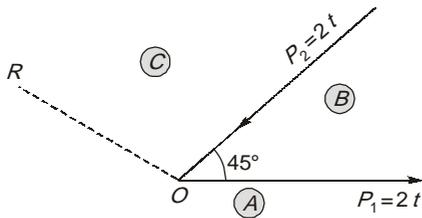
From the force diagram the force  $R$  to be applied at  $O$  in order to keep the body in equilibrium is given by
