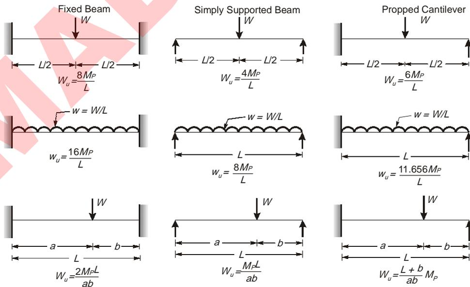
Ratio of collapse load of propped cantilever beam to the simply supported beam is  $\frac{11.656}{8} = 1.457$
