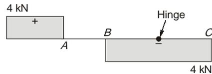
$\therefore$  BM at A =  $4 \times 2.5 = 10\text{ kN-m}$
