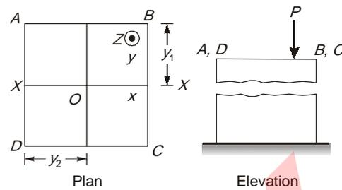
If the compressive stresses are taken as positive and area  $A = 2y_1 \times 2y_2 = 4y_1 y_2$  and the moment of inertia about X and Y axis being  $I_{xx}$  and  $I_{yy}$  respectively, then the stress at the corner D is
