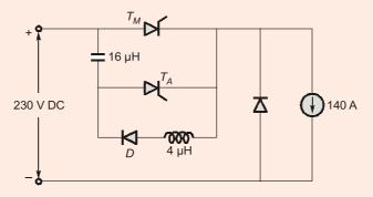
where  $T_{\rm M}$  is main thyristor and  $T_{\rm A}$  is Auxiliary thyristor.
