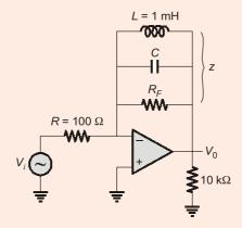
Assume resonant frequency of parallel RLC network as 32 kHz
