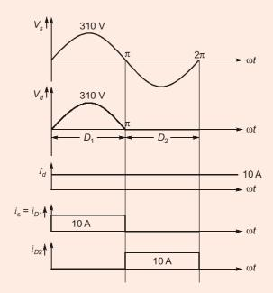
$$V_{d,\text{avg}} = \frac{1}{2\pi} \int_{0}^{\pi} V_{m} \sin\omega t \cdot d(\omega t) = \frac{V_{m}}{\pi} = \frac{310}{\pi} = 98.67 \text{ V}$$
