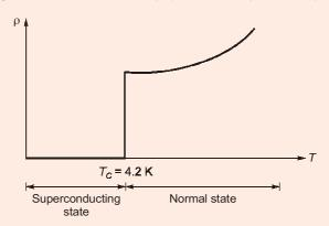
There is an abrupt change in resistivity of mercury at critical temperature ( $T_c$ ). Pure superconductors are type-I superconductors and following figure represents comparison of resistivity of pure superconductor and normal metal.
