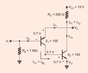
$$\begin{split} V_o &= 0.7 + V_{\text{in}} \\ V_{\text{in}} &= I_{B1} \times R_B \\ &= 10^6 I_{B1} \\ \\ &= 10^6 \frac{I_{E1}}{(1+\beta_1)} \\ \\ &= 10^6 \times \frac{I_{E1}}{100} \\ \\ &= 10^4 I_{E1} \implies V_o = 0.7 + 10^4 I_{E1} \\ V_o &= V_{CC} - (I_{E1} + I_{C2}) R_C \\ \\ &= V_{CC} - (I_{E1} + \beta_2 I_{B2}) R_C \\ \\ &= V_{CC} - (I_{E1} + \beta_2 I_{C1}) R_C \\ \\ &= V_{CC} - (I_{E1} + \beta_2 I_{E1}) R_C \\ \\ &= V_{CC} - (I_{E1} + \beta_2 I_{E1}) R_C \end{split}$$
