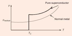
Impure superconductors are type-II superconductors and following figure represents comparison with normal metal.
