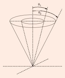
Calculate the angle  $\theta$  at which the voltage is 75 volts. Assume air as the dielectric in the region between the two coaxial cones.
