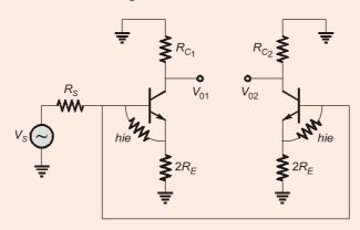
$$\begin{split} \frac{V_{o1}}{V_s} &= \frac{-h_{fe}I_bR_c}{2I_bR_s + h_{ie}I_b + (1 + h_{fe})I_b \times 2R_E} \\ \frac{V_{o1}}{V_s} &= \frac{-h_{fe}R_{c1}}{2R_s + h_{ie} + 2(1 + h_{fe})R_E} \\ \frac{V_{o2}}{V_s} &= \frac{-h_{fe}R_{c2}}{2R_s + h_{ie} + 2(1 + h_{fe})R_E} \end{split}$$
