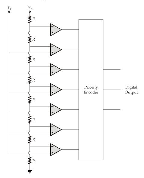
The 3-bit flash type ADC consists of a voltage divider network having 7 comparator and a priority encoder.
