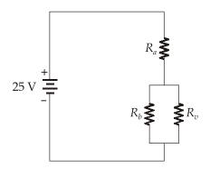
$$R_{\text{eq}} = R_b \parallel R_v$$
