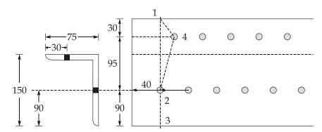
Length of gusset plate required =  $5 \times 50 + 2 \times 40 = 330 \text{ mm} < 350 \text{ mm}$  (O.K) Net area along 1-2-3,  $A_{n1} = (215 - 22) \times 10 = 1930 \text{ mm}^2$
