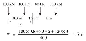
Now, the absolute maximum bending moment will occur either under the 100 kN or the 80 kN load, when the respective load and the resultant of the load system is placed equidistant from the mid-span of the girder.
