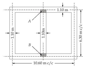
Total centre length of wall =  $2 \times c/c$  length of long wall +  $3 \times c/c$  length of short wall
