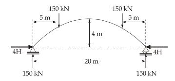
$$4H = \frac{\int_{0}^{1} \frac{\overline{EI}}{EI}}{\int_{0}^{20} \frac{y^{2} dx}{EI}} \left[ y = \frac{4h}{l^{2}} x(l-x) \right]$$
