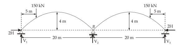
Now, we can again use symmetry to calculate the value of 2H corresponding to the given loading condition.
