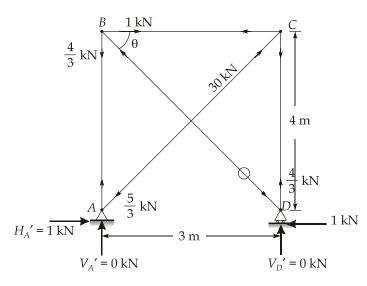
Let  $V_A{'}$  and  $H_A{'}$  be the vertical and horizontal reactions at A respectively and  $V_D{'}$  be the vertical reaction at D.
