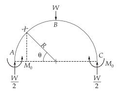
Let us assume reacting moments  $M_0$  is acting at A and C and upward reaction at A and C be  $\frac{W}{2}$  each.
