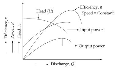
**Constant Efficiency Curve**: For obtaining constant efficiency curve, the head versus discharge curves and efficiency versus discharge curves for different speeds are used. By combining these curves ( $H \sim Q$  curves and  $\eta \sim Q$  curves), constant efficiency curves are obtained.
