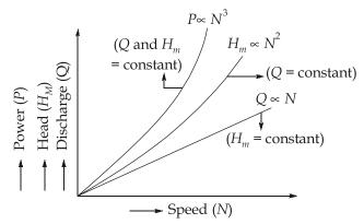
**Operating Characteristic Curves**: If the speed is kept constant, the variation of manometric head, power and efficiency with respect to discharge gives the operating characteristics of the pump.
