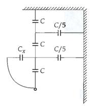
Calculate the voltage on line-end unit and the value of capacitance  $C_X$ .
