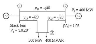
Using Newton-Raphson method, start with the initial guess of  $V_2^{(0)} = 1.05 + j0$  and  $V_3^{(0)} = 1.0 + j0$  and keeping  $|V_2| = 1.05$  pu, determine the phasor values of  $V_2$  and  $V_3$  after one iteration.
