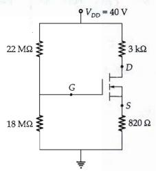
If  $V_{GS(TH)}$  = 5 V,  $I_{D(ON)}$  = 3 mA at  $V_{GS(ON)}$  = 10 V, then determine  $I_{DQ}$ ,  $V_{GSQ}$  and  $V_{DS}$ . [20 marks]
