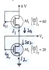
If both transistor have parameters  $\mu_n C_{ox}$  = 40  $\mu$ A/V² and  $V_{Th}$  = 0.9 V then calculate the output voltage  $V_o$ .
