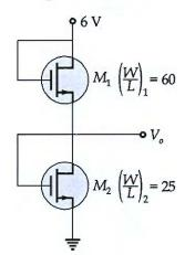
If both transistor have parameters  $\mu_n C_{ox}$  = 40  $\mu A/V^2$  and  $V_{Th}$  = 0.9 V then calculate the output voltage  $V_a$ .
