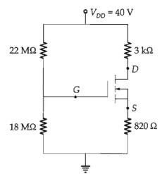
If  $V_{GS(\mathrm{TH})}$  = 5 V,  $I_{D(\mathrm{ON})}$  = 3 mA at  $V_{GS(\mathrm{ON})}$  = 10 V, then determine  $I_{DQ}$ ,  $V_{GSQ}$  and  $V_{DS}$ .
