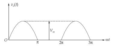
$\therefore a_o = dc$  component of output voltage,
