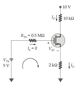
Apply KVL in Gate-source loop
