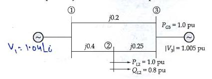
Compute  $V_1$ ,  $V_2$  and  $V_3$  upto one iteration.
