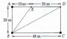
If A is a benchmark having an elevation of 120 m, calculate the correct elevations of B and C. Also find the missing staff reading at C from instrument location E.
