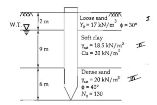
The angle of friction between pile and soil is 0.75 times of angle of internal friction of soil. The earth pressure coefficient for loose sand is 1 and for dense sand is 2. Adhesion factor for soft clay is taken as 1.
