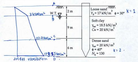
The angle of friction between pile and soil is 0.75 times of angle of internal friction of soil. The earth pressure coefficient for loose sand is 1 and for dense sand is 2. Adhesion factor for soft clay is taken as 1.
