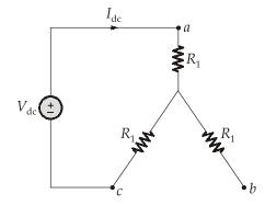
$$2R_1 = \frac{V_{dc}}{I_{dc}} = \frac{9.07}{28} = 0.3239$$
