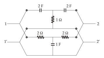
The total Y-parameters of the network is obtained by addition of two individual sub-network Y-parameter.
