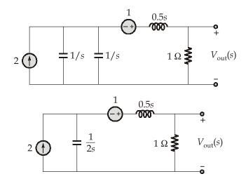
Apply source transformation and combine series voltage source to produce a series circuit.
