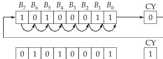
4. **RCL** : This instruction is used to rotate the data byte/word toward the left through carry.
