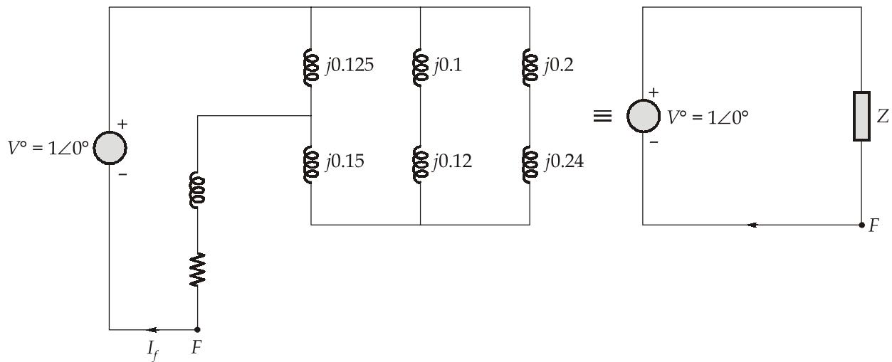
Assuming no-load prefault conditions, i.e., prefault currents are zero. Post-fault current can be calculated by the circuit model as shown.
