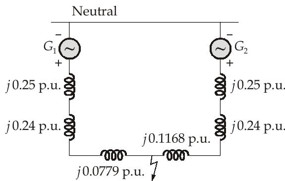
$$\begin{aligned} X_{\text{eq (p.u.)}} &= j(0.25 + 0.24 + 0.0779) \parallel j(0.25 + 0.24 + 0.1168) \text{ p.u.} \\ &= j0.5679 \parallel j0.6068 \text{ p.u.} \\ &= \frac{j0.5679 \times j0.6068}{j0.5679 + j0.6068} = j0.2934 \text{ p.u.} \end{aligned}$$
