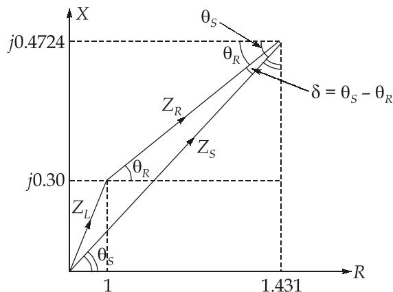
(iii) Based on diagram,  $\vec{Z}_S$  can be obtained analytically or graphically,
