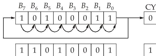
3. **RCR** : This instruction is used to rotate the data byte/word towards the right through carry.
