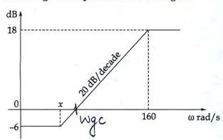
Find the transfer function and gain cross-over frequency.
