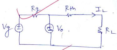
Where  $V_0 = 0.125 \text{ Vg} = 1.5 \text{ Volts}$ . Rg = R + 10052.
