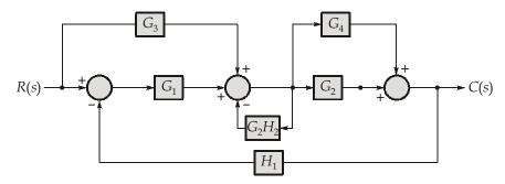
**Step-2**: Eliminate the inner feedback path and combine the blocks in parallel.
