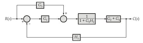
**Step-3**: Move the summing junction on the right of the block  $G_1$  to its left and combine the blocks in cascade.
