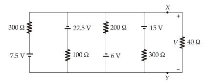
$$V_{\text{th}} = V_{XY} = \frac{\frac{7.5}{300} - \frac{22.5}{100} - \frac{6}{200} + \frac{15}{300}}{\frac{1}{300} + \frac{1}{100} + \frac{1}{200} + \frac{1}{300}}$$
