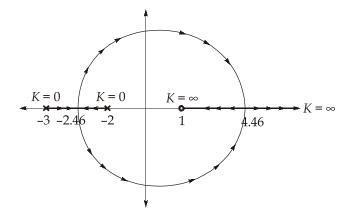
(iii) Smallest settling time will occur when both roots are as far away as possible to the left of  $j\omega$ -axis. Using magnitude condition,
