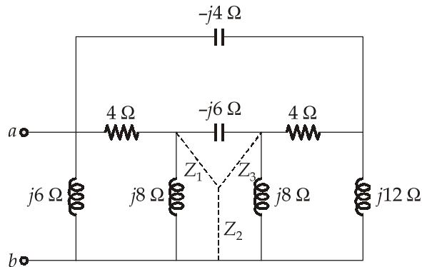
Transform the delta connection to star connection as shown in figure.
