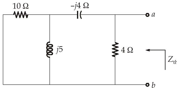
$$\begin{aligned} Z_{th} &= 4 \parallel (-j4 + (10 \parallel j5)) \\ &= 4 \parallel (-j4 + 2 + j4) \end{aligned}$$
