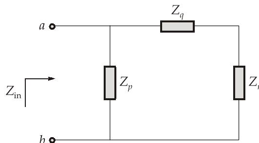
$$\begin{aligned} Z_{\text{in}} &= Z_p \parallel (Z_q + Z_r) \\ &= (0.68 + j3.62) \parallel (0.20 - j2.75 + 1.38 + j5.07) \\ Z_{\text{in}} &= (0.66 + j1.48) \Omega \end{aligned}$$
