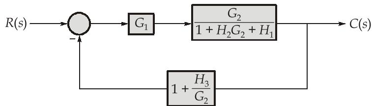
**Step 4 :** Combining the two blocks in cascade and eliminate the feedback path.
