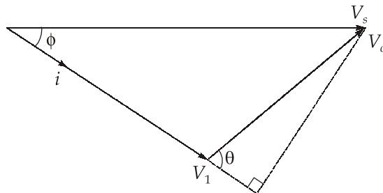
$$V_s^2 = V_1^2 + V_o^2 + 2V_1 V_o \cos \theta$$
