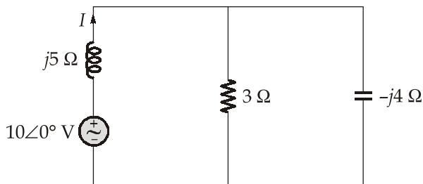
$$\begin{aligned} I' &= \frac{10\angle 0^\circ}{j5 + (3 \parallel -j4)} = \frac{10\angle 0^\circ}{j5 + 2.4\angle -36.86^\circ} \\ &= 2.47\angle -61.66^\circ \text{ A} \end{aligned}$$
