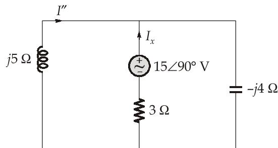
$$\begin{aligned} I_x &= \frac{15\angle 90^\circ}{3 + (j5 \parallel -j4)} = \frac{15\angle 90^\circ}{3 - j20} \\ I_x &= 0.7417\angle 171.46^\circ \text{ A} \end{aligned}$$
