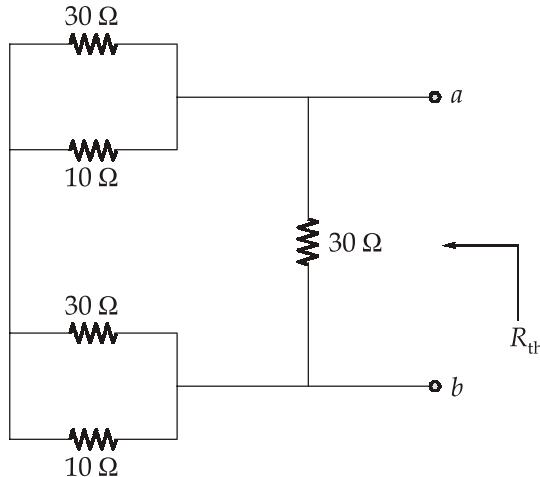
$$\begin{aligned} R_{th} &= 30 \parallel (30 \parallel 10 + 30 \parallel 10) \\ &= 30 \parallel (7.5 + 7.5) = 30 \parallel 15 = 10 \Omega \end{aligned}$$
