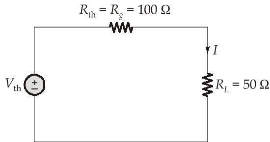
$$V_{\text{th}} = V_s = 0.125V_g = 1.5 \text{ V}$$
