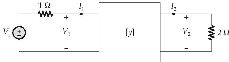
$$V_s = V_1 + I_1 \quad \text{or} \quad V_s - V_1 = I_1 \quad \dots(3)$$
