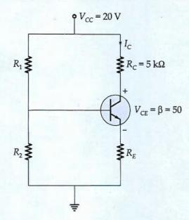
The operating point is Q(11.5 V, 1.5 mA). For stability factor  $S \le 2$ , determine the values of  $R_1$ ,  $R_2$  and  $R_E$ .
