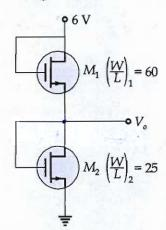
If both transistor have parameters  $\mu_n C_{ox} = 40 \,\mu\text{A/V}^2$  and  $V_{Th} = 0.9 \,\text{V}$  then calculate the output voltage  $V_o$ .
