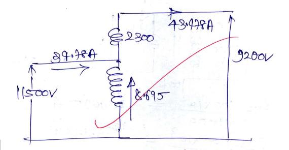
Voltage Ratio = 9200 = 4 11500 = 5 FUA output = 43.978 x 9200 = 400 KVA
