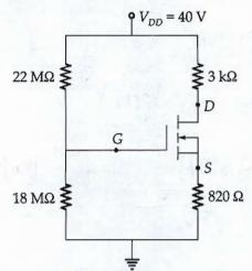
If  $V_{GS(TH)} = 5 \text{ V}$ ,  $I_{D(ON)} = 3 \text{ mA}$  at  $V_{GS(ON)} = 10 \text{ V}$ , then determine  $I_{DQ}$ ,  $V_{GSQ}$  and  $V_{DS}$ .
