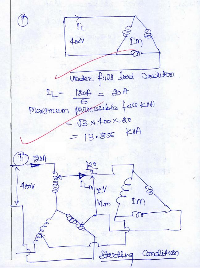
Far 60% Japping, Leve valtage to motor= 600/ X 400V = 240 V Starting Rino awarent to topoto = 120A = 200 A fell load line current to motor = 200A Sex tenses = 83.33A full load KVA = 13 x 290 x x 33.33 A = 13.856 KM 190 = 20A VAC = 200V [L-1) forwA= 13 X 400 X 20 = (13.850 PUA
