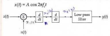
The low pass filter has unity gain in the passband and bandwidth W, where  $f_c < W$ . The noise n(t) is white with two sided power spectral density  $\frac{1}{2}N_0$ . Determine the signal to noise ratio at the output y(t).
