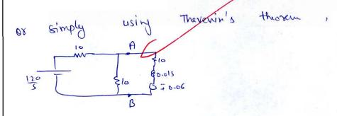
$$V_{\text{th}}_{AB} = \frac{120}{5} \times \frac{10}{10+10} = \frac{60}{5}$$
