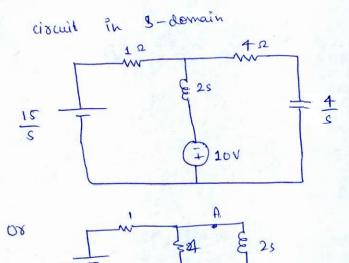
$V_{L} = L \ell(0^4)$   $= 2 \times 5 = 10 \text{V}$
