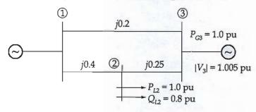
Compute  $V_1$ ,  $V_2$  and  $V_3$  upto one iteration.
